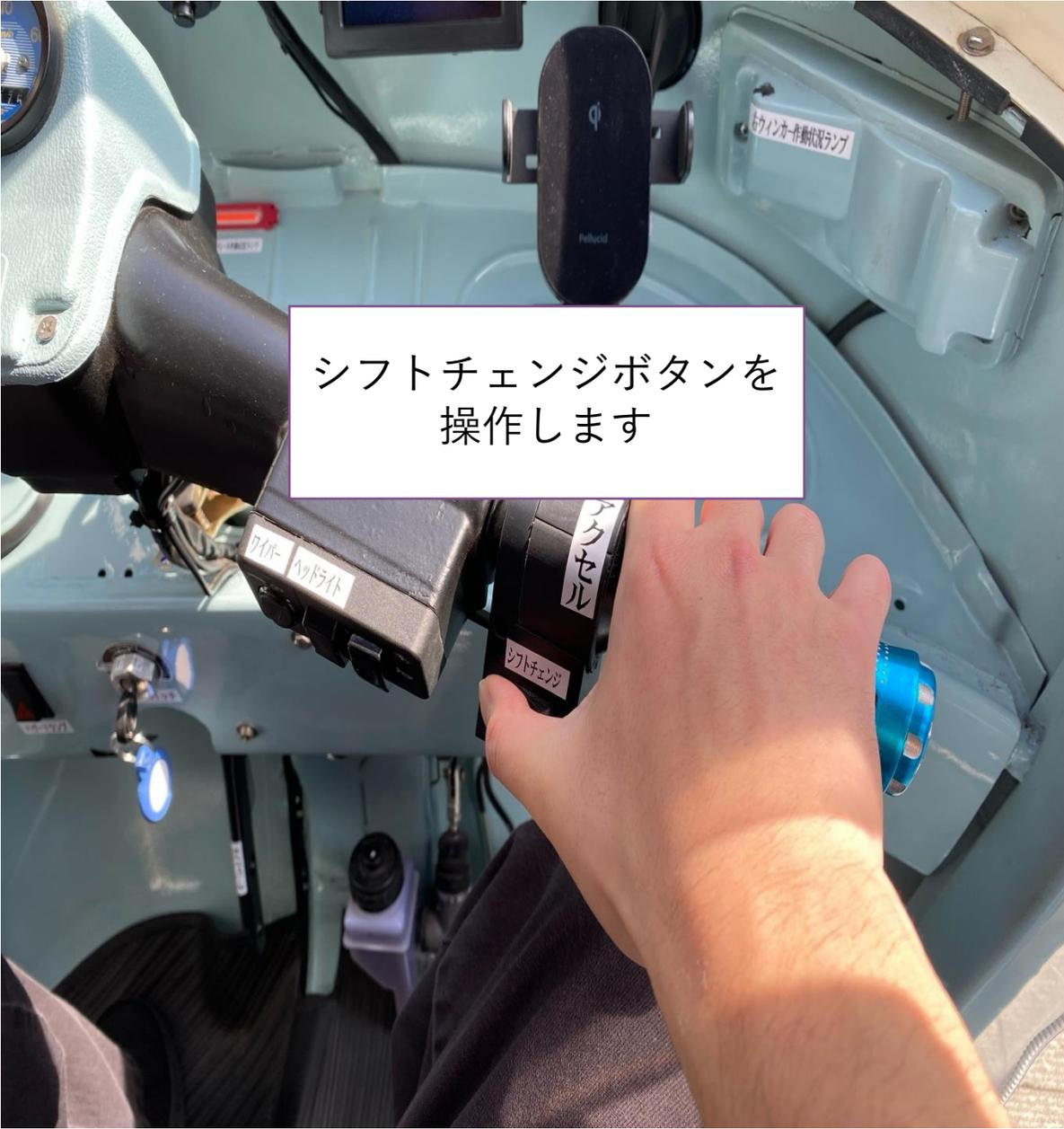
A close-up photograph of a person's hand operating a control panel. The hand is pressing a button labeled 'シフトチェンジ' (Shift Change). To the left, there is a control unit with labels 'ワイパー' (Wiper) and 'ヘッドライト' (Headlight). Above the hand, there is a black lever labeled 'アクセル' (Accelerator) and 'セル' (Start). The background shows the interior of a vehicle with a light blue dashboard and various controls.
