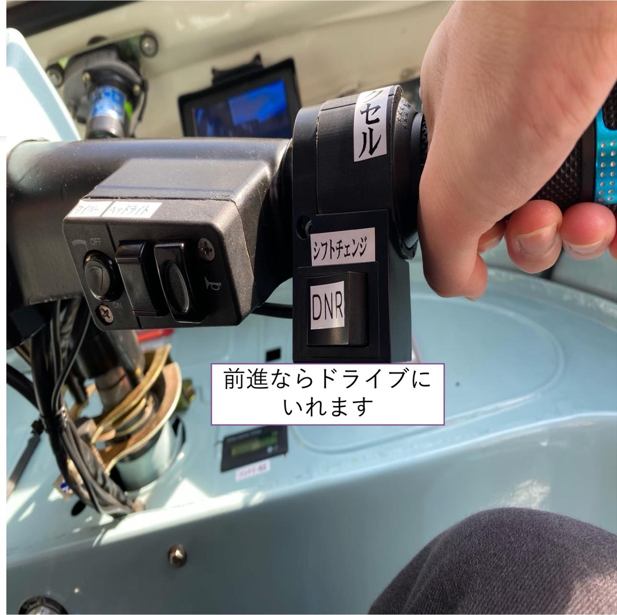
A close-up photograph of a hand operating a drive mode selector. The hand is moving a lever labeled 'セル' (Start) and 'シフトチェンジ' (Shift Change). Below the lever, there is a button labeled 'DNR'. The background shows the interior of a vehicle with a light blue dashboard and various controls.
